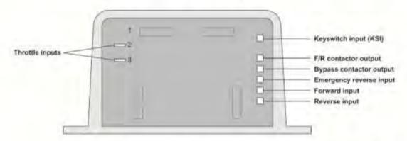
Several manufacturers make mating connectors that fit this connector. The part numbers listed are for the recommended 0.75 mm<sup>2</sup> (#18 AWG) vinyl insulated stranded wire.
