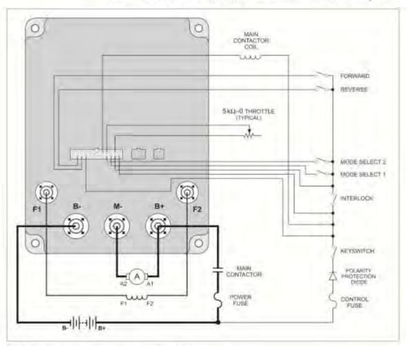
Fig. 3 Standard wiring configuration. Carris PMC 1244 controller.
