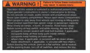
When a disconnect handle is installed, this label is required (located in front of handle): # 4800012J
