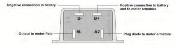
The cables used for the battery and motor connections must be heavy enough to carry the high current required. Rubber insulated welding cable is convenient to work with because of its flexibility.
