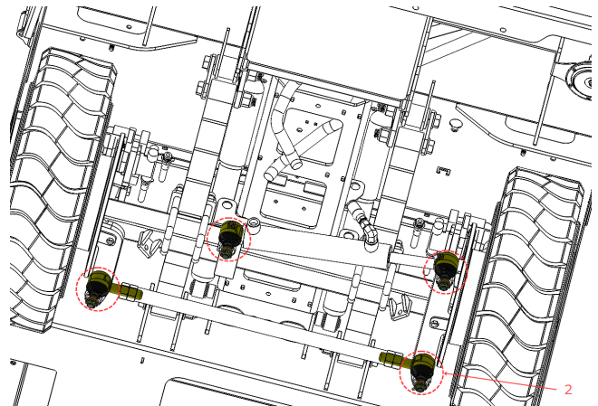
Figure 32. Tie Rods Ends Inspection.
