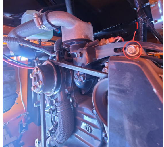
Figure 35. Belt Tension Adjustment.
