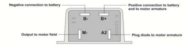
The cables used for the battery and motor connections must be heavy enough to carry the high current required. Rubber insulated welding cable is convenient to work with because of its flexibility.
