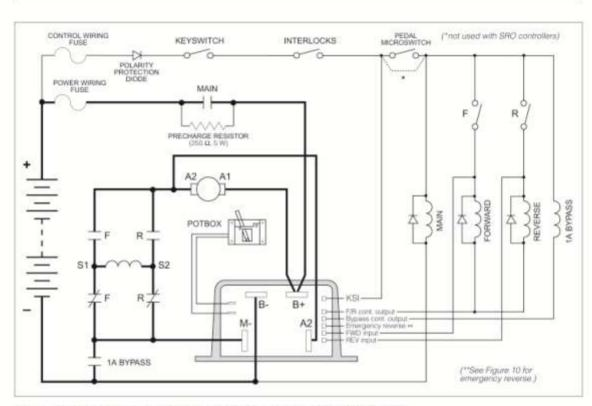
Fig. 8 Basic wiring configuration, Curtis PMC 1204X/1205X/1209/1221 controllers.
