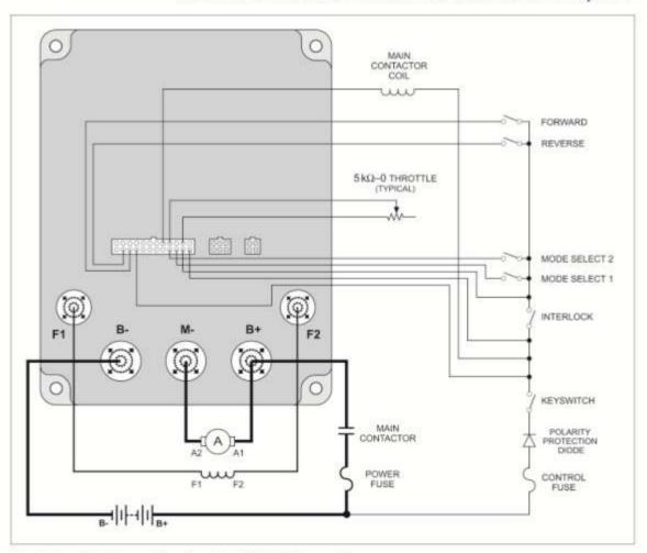
Fig. 3 Standard wiring configuration, Curtis PMC 1244 controller.
