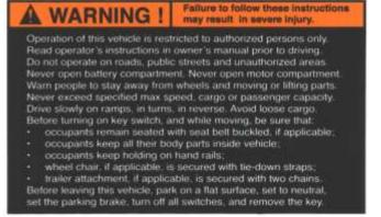
When a disconnect handle is installed, this label is required (located in front of handle): # 4800012J
