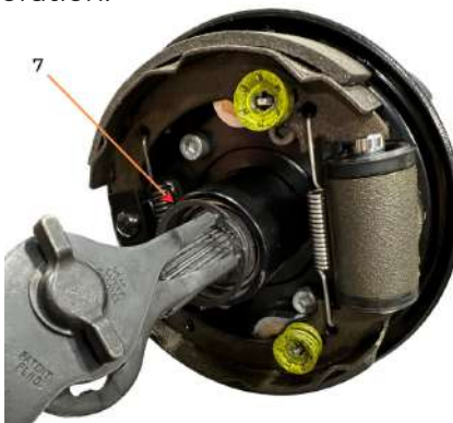
Figure 59. Circlip and Axle Shaft Removal.
