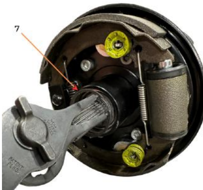
Figure 55. Circlip and Axle Shaft Removal.
