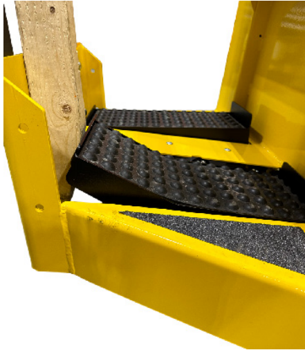
Figure 55. Master Pedal Blocking Illustration.
