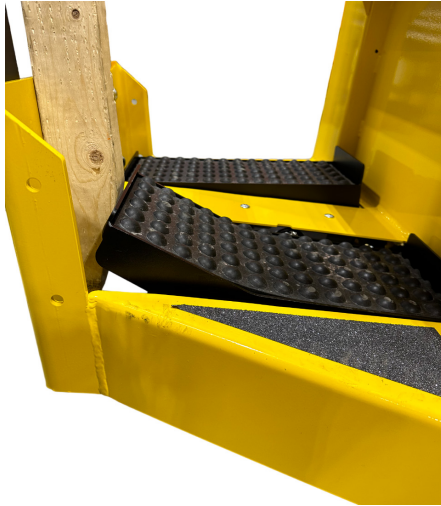
Figure 55. Master Pedal Blocking Illustration.
