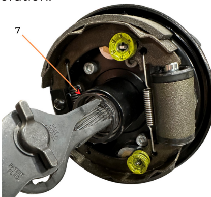
Figure 59. Circlip and Axle Shaft Removal.
