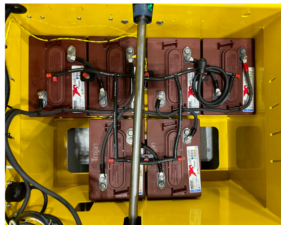
Figure 62. Batteries Watering System.
