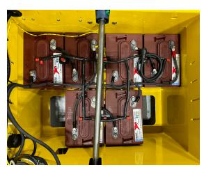
Figure 63. Batteries Watering System.
