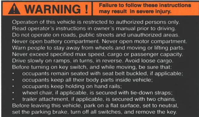
When a disconnect handle is installed, this label is required (located in front of handle):
