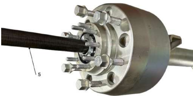
Figure 49. Rear Axle Shaft Removal.
