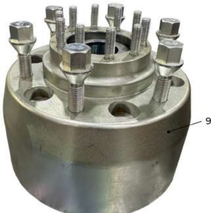
Figure 52. Wheel Studs and Brake Drum Removal.
