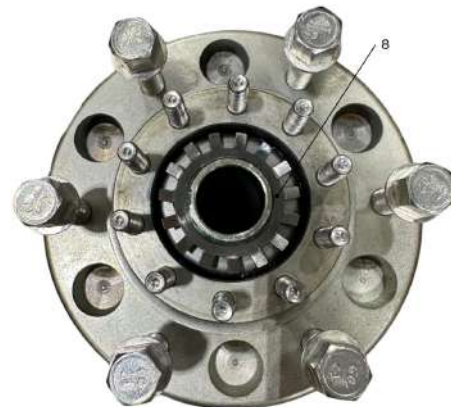
Figure 51. Axle End Lock Removal.
