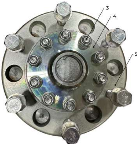
Figure 61. Bolts, Axle Hub Cap and Brake Drum Removal.
