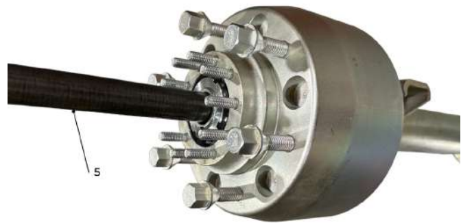
Figure 65. Rear Axle Shaft Removal.
