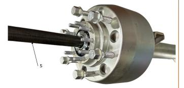
Figure 49. Rear Axle Shaft Removal.
