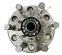
Figure 51. Axle End Lock Removal.
