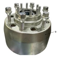
Figure 52. Wheel Studs and Brake Drum Removal.
