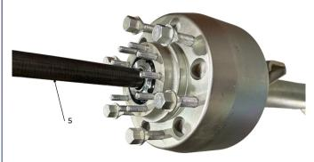
Figure 65. Rear Axle Shaft Removal.
