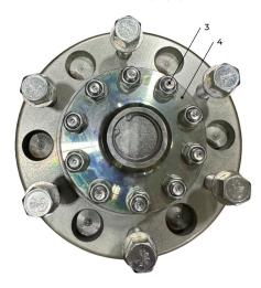
Figure 64. Bolts and Axle Hub Cap Removal.
