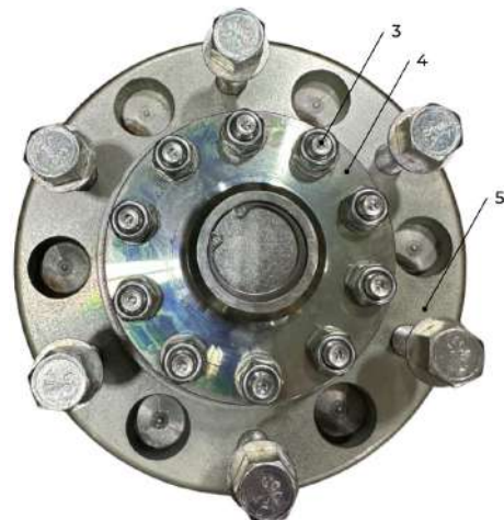
Figure 77. Bolts, Axle Hub Cap and Brake Drum Removal.
