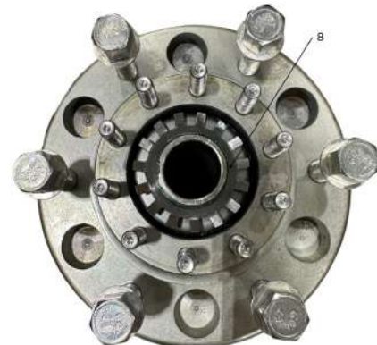
Figure 61. Axle End Lock Removal.
