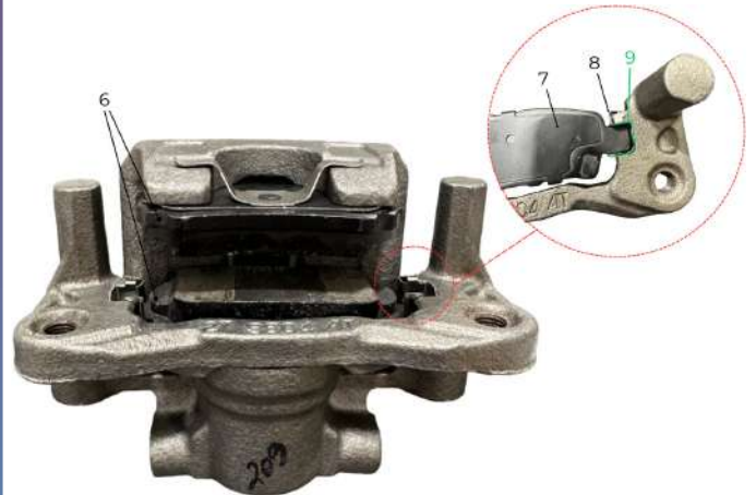
Figure 43. Brake Pads and Shims Inspection.
