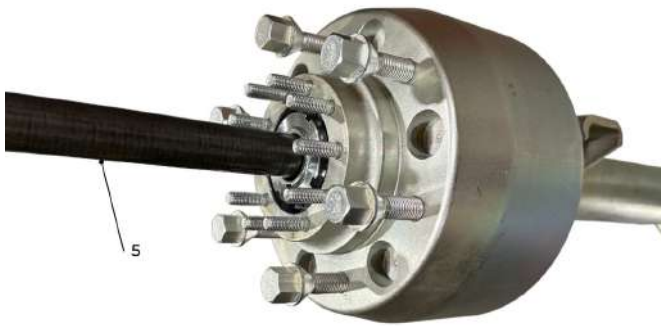
Figure 85. Rear Axle Shaft Removal.
