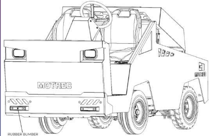
Figure 31. Rubber Bumper Inspection.
