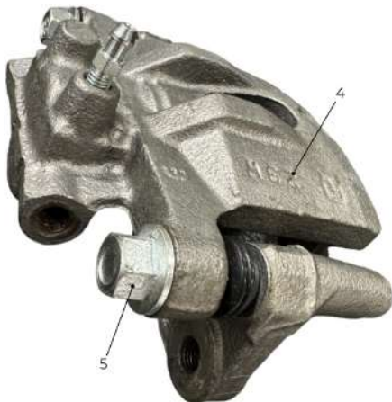
Figure 42. Slide Pins and Caliper Removal.
