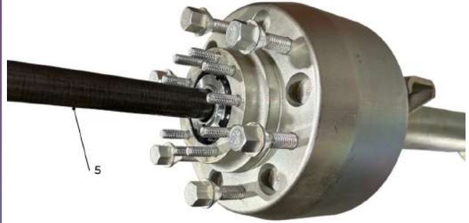
Figure 59. Rear Axle Shaft Removal.
