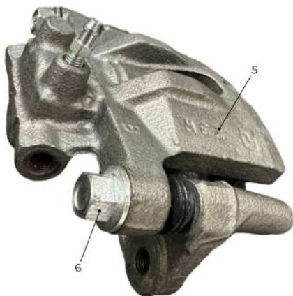
Figure 53. Slide Pins and Caliper Removal.
