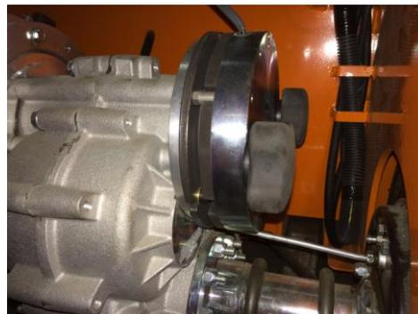
When the vehicle is ready to be used, the knobs must be removed from the electromagnetic brake and put back to their storage location.
