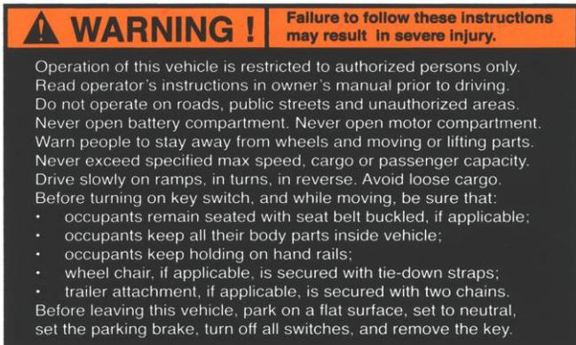
When an emergency push button is installed, this label is required (located under push button): # 3109800006
