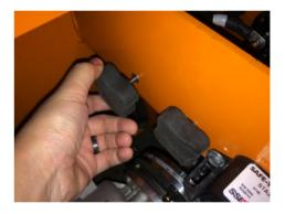
2- Screw the knobs behind the electromagnetic brake to manually release the brake.
