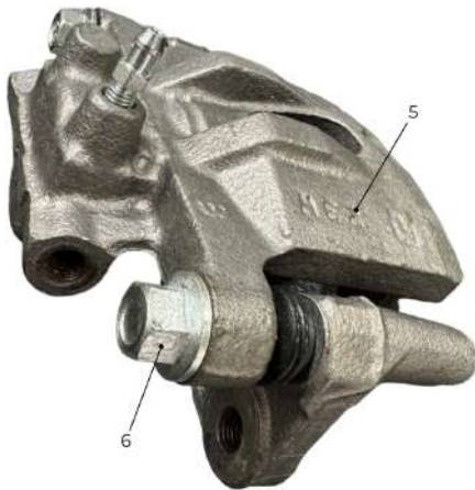
Figure 58. Slide Pins and Caliper Removal.
