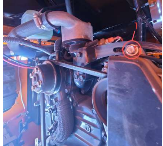
Figure 34. Belt Tension Adjustment.
