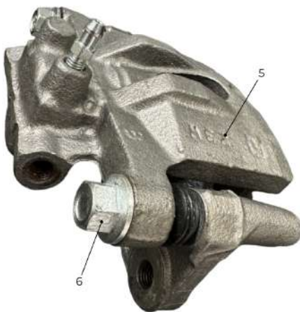
Figure 43. Slide Pins and Caliper Removal.
