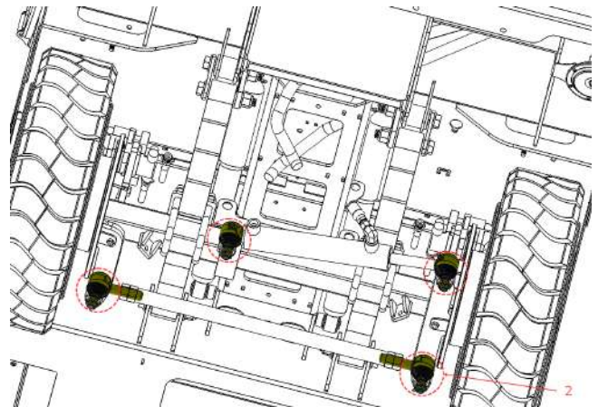
Figure 31. Tie Rods Ends Inspection.
