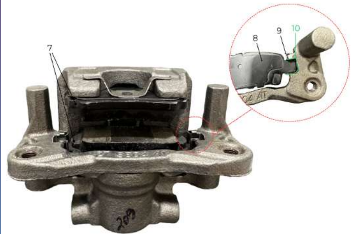
Figure 44. Brake Pads and Shims Inspection.
