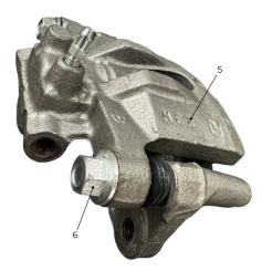
Figure 43. Slide Pins and Caliper Removal.
