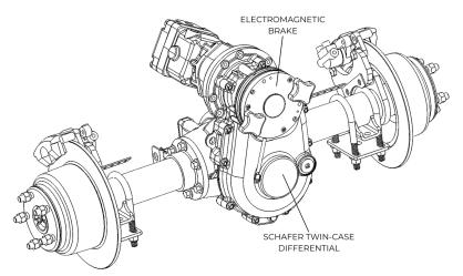
Figure 6. Heavy Duty Differential.
