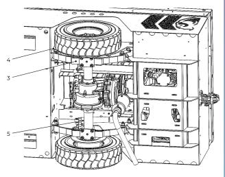
Figure 28. Rear Suspension And Shock Absorbers Inspection.
