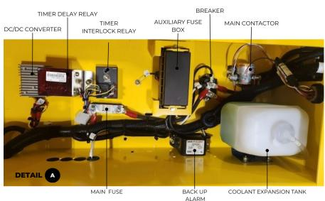
Figure 2. a. Electrical System Compartments (View A).
