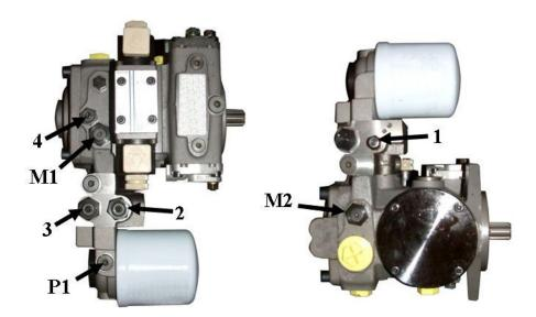
Figure 69. Hydrostatic Pump Adjustement.
