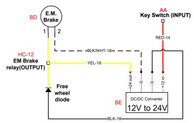
Figure 70. DC/DC Converter Input and Output Terminals Inspection.
