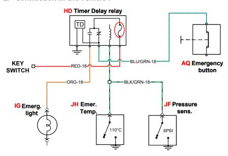
Figure 3. Timer Delay Annunciator Connection - Electrical Diagram-.
