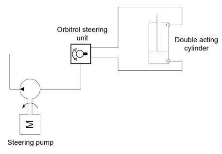
Figure 68. Hydraulic Steering System.
