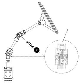
Figure 30. Universal Joint Inspection.
