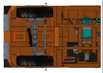
Figure 64. Distance between the front tires.
