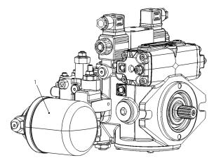
Figure 24. Hydrostatic Pump Oil Filter Replacement.
