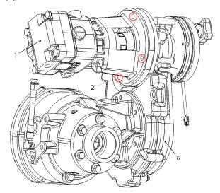
Figure 54. Removing screws.
