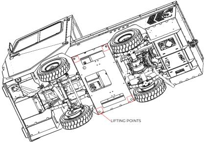
Figure 20. Lifting Points.
