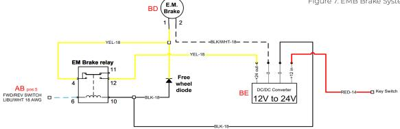
Figure 8. EMB Connection - Electrical Diagram -.
