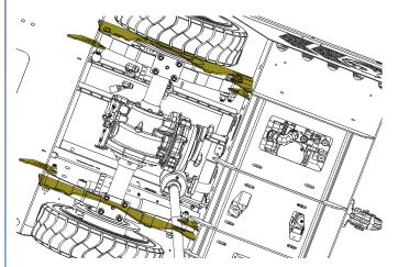
Figure 40. Rear Suspension Mounting Tabs.
