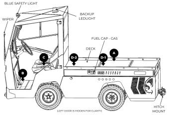
Figure 16. General Components (Detail A, B and C).
