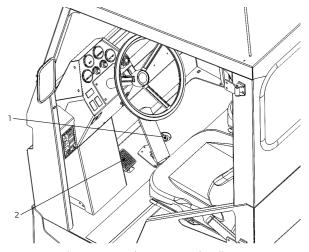
Figure 60. Brake System Bleeding.
