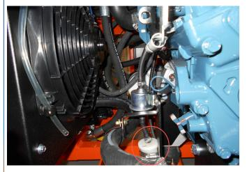
Figure 35. Location of the Fuel Filter In the Gas Engine.
