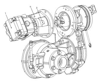
Figure 55. Disconnecting Motor, coupling 7/8 and motor-differential adapter.
