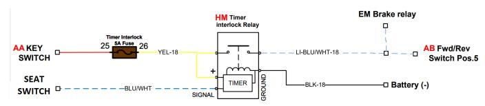
Figure 4. Adjustable Timer Interlock Delay Connection - Electrical Diagram-.
