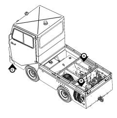
**NOTE**: The vehicle's frame is to be considered as a ground.
