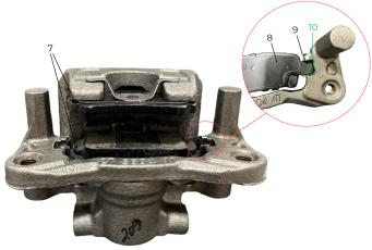
Figure 44. Brake Pads and Shims Inspection.
