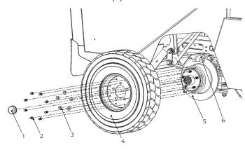
Figure 57. Wheel Removal.
