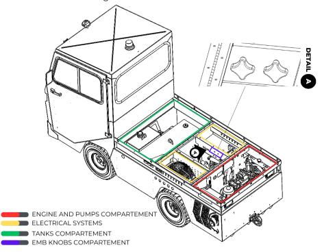
Figure 1. Equipment Compartments.
