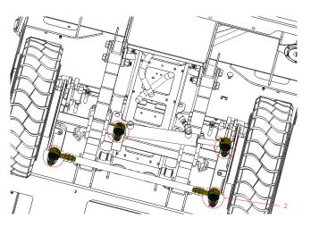
Figure 31. Tie Rods Ends Inspection.
