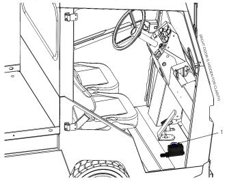
Figure 21. Front Fluid Leaks In The Master Cylinder.
