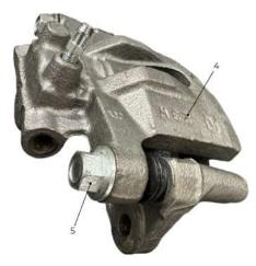
Figure 40. Slide Pins and Caliper Removal.
