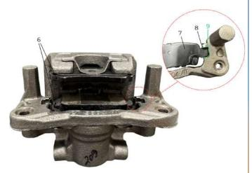
Figure 41. Brake Pads and Shims Inspection.
