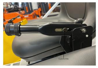
Figure 44. Clevis Pin Position.
