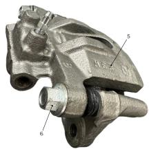
Figure 47. Slide Pins and Caliper Removal.
