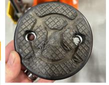
Figure 20. Jack Rubbers Used For Lifting
