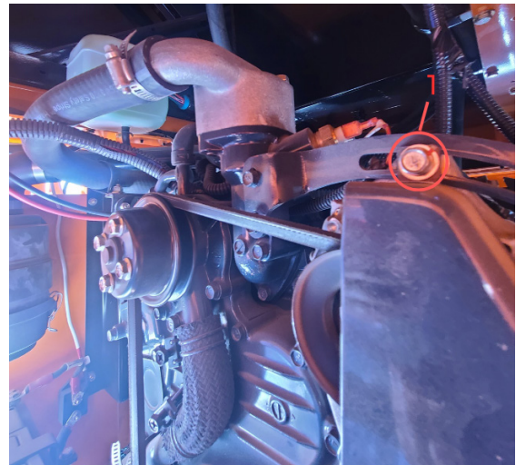
Figure 29. Belt Tension Adjustment.
