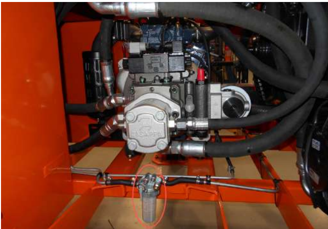
Figure 38. Location of the Fuel Filter In a Diesel Engine.
